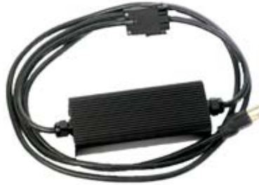
DPP120 power in-feed with sensor and 10 ft power cord with standard NEMA 5-15P 15 amp plug on one end and 3-port connector plug on the other end.
